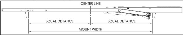
• Mount the rack to each foot using four 3/8" x 1" hex heads, four 3/8" split lock washers and four 3/8" flat washers. The same slot should be used at each location.
