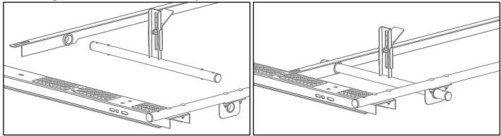
Ladder clamp on the clamp tube is adjustable. When finished installing rack, clamp must be adjusted to fit firmly against ladder.
