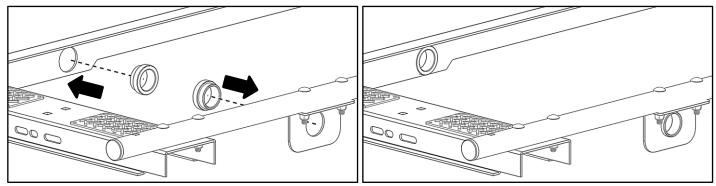
Insert clamp tube into both plastic bushings in the orientation shown. Be sure to install the bushings in an orientation so they CANNOT fall out.
