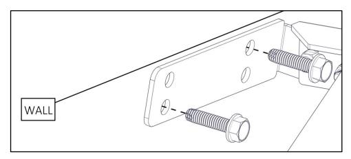
Note: If desired, one can attach this bracket using 1/4" x 7/8" hex head bolts, 1/4" flat washers and 1/4" flanged nyloc nuts. This provided a more robust fitment, but is more difficult to install.
