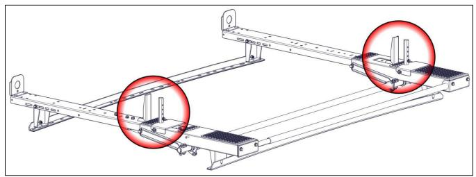
NOTE: In the rare instance the upper location on the front bow needs to be used, a 3/8" bolt and lock nut will need to be used to install the ladder stop.
