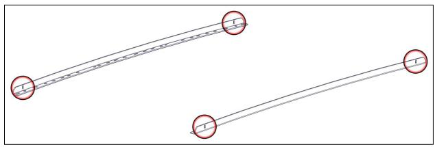
• Using 5/16" x 1" carriage bolts, 5/16" flat washers and 5/16" lock nuts, bolt the foot to the mount rail in the orientation shown.
