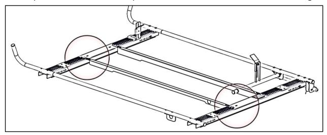
• Insert plastic bushings into the clamp and lock L bracket and the hanger bracket installed in Step 2, with flanges as shown so they cannot come out at a later time. If bushings are not placed in correct orientation, they can fall out.
