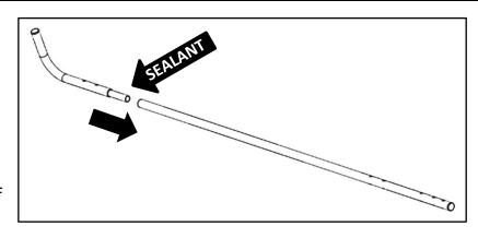
• Be sure the bend is towards the front and to the outside of the vehicle as shown.
