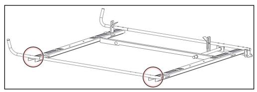
• Mount the tube assembly to the bows using 5/16" x 2" carriage bolts, 5/16" flat washers and 5/16" lock nuts.
