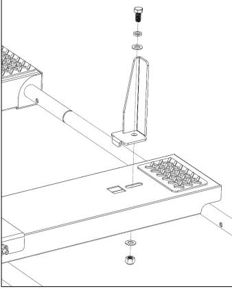
• Gently set and hold the ladder in position on the rack, as shown, and adjust the stepladder pan into position.
