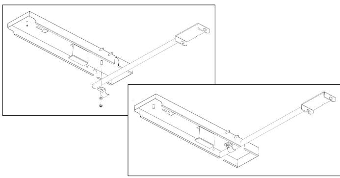
• Attach pan support tube assembly to the pan of the drop down ladder rack, to the right, on the 5/16" studs that are closest to the center of the vehicle.
