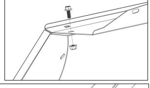
• Using a 1/4" x 5/8" flanged bolt and 1/4" flanged lock nut, bolt corner panel to side wing.
